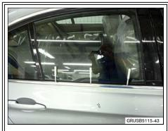
1. Use plastic wedges to create a gap between the window and the weatherstrip.
