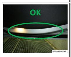
3. Check the door panel for water drops near the bottom by looking in from the left side door. If no water leaks can been seen, no further work is required
