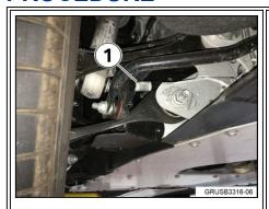
1. Raise the vehicle to access the parts label on the left rear axle (1).
