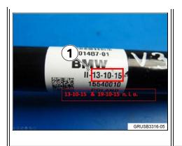
2. Inspect the date code on the left rear output shaft (DD-MM-YY) (1). Is the production date code either 13-10-15 OR 19-10-2015?
