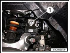
(i3 Rex only) Replace the screw for the right side motor mount (1).
