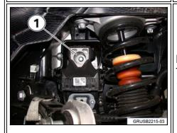
Replace the screw for the left side motor mount (1). Tightening: Jointing torque 96 Nm, angle of rotation 120°
