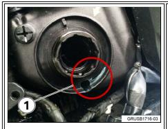
Coolant expansion tank leak in the vicinity of the drainage channel. (1)
