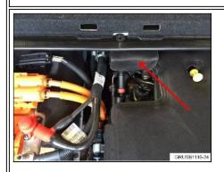
It is recommended that prior to removal of the oil cap, the service flap be folded behind the edge of the engine compartment (as shown on the picture) to provide unobstructed access to the oil filler neck.
