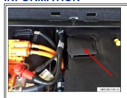
The service flap of the engine sound insulation covers the oil filler neck and the filler cap.
