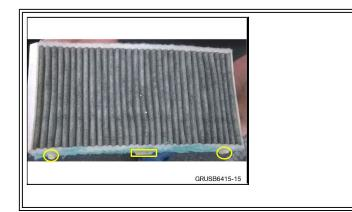
6. Allow the applied glue time to dry then then install the upper and lower micro-filters in the housing (REP 64 31 010).
