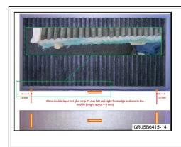
All 3 hot glue applications must be double layered, be 15 mm long and have a total height of 4-5 mm. Placement of the hot glue must be in the exact locations shown to prevent complications with condensate water flow.
