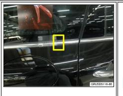
Check the rubber strip on the trim below the fixed rear window. Is the rubber strip cracked? YESreplace the trim strip following REP 51 36 040 "Removing and installing/replacing strip on rear left or right side window". NO- Go to next step 2.
