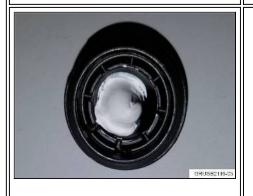
5. Grease the socket for the piston rod end, in the thrust piece, with lubricant specified below.
