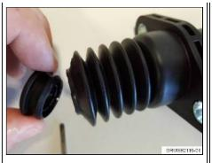
3. Disassemble thrust piece of the clutch slave cylinder from the piston rod of the clutch slave cylinder.
