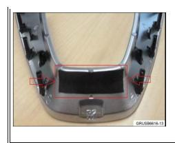
4. Reinstall the steering wheel cover according to REP 3233016 "Cover for sports steering wheel".
