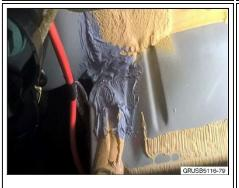
View of the battery box from below with the rework.
