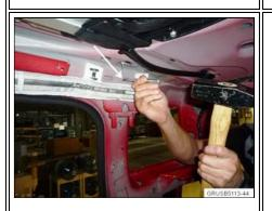
4. Insert a steel center punch through the rear rectangle opening of the reinforcement. Using a heavy steel hammer, hit the punch hard enough to create a small dimple in the sheet metal.
