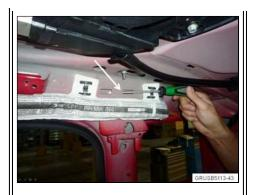
applying varying pressure to the metal roof support as shown. If the noise can be eliminated by applying pressure, proceed to the next step
