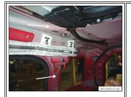
2. Remove the headliner and inner C-pillar trim from the affected side. Refer to REP "RA 51 44 013 Removing and installing/replacing headlining".
