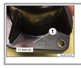
Although the improved vehicle wiring harness has the same part number, it can be identified by the index (1) at the rear of the part number. (2) indicates the last 7 digits of the part number.
