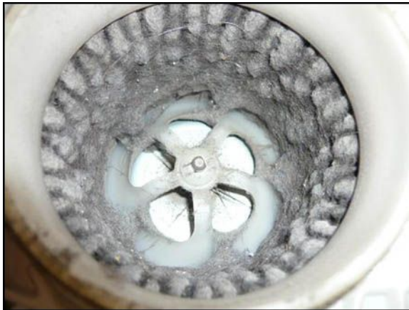
Figure 1. HV Battery Cooling Fan BEFORE Cleaning
