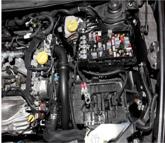
***Fig. 8 Battery Removal***
