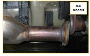
• Remove the nuts holding the front exhaust pipe onto the cylinder heads. Retain these nuts for use at reassembly.
