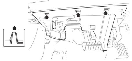
Remove the necessary screws, release the claws and disconnect the harness connectors from the switches before CAREFULLY removing the instrument panel lower trim cover.
