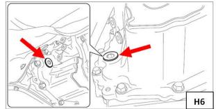
The CVT fluid level is correct when it is up to bottom of the filler plug hole.
