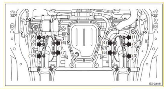
Reconnect the A/F and O2 Sensor wiring harness connectors.
