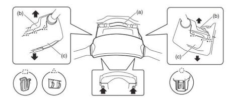
After disconnecting all the wiring harness connectors, CAREFULLY remove the roll connector, steering angle sensor and the combination switch assemblies. IMPORTANT: Do not disturb the postion of the roll connector while removed from the steering column. As shown in the photo, use a piece of tape to keep it in alignment while removed.
