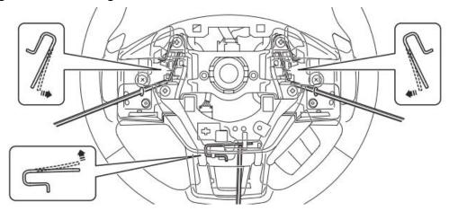
• CAREFULLY, release / remove the 2 airbag module harness connectors and set the module aside in a safe place.
