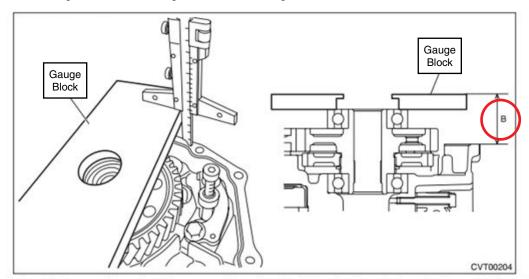
3) Obtain the thickness of transfer driven gear shim using the following formula to select zero to three transfer driven gear shims.
