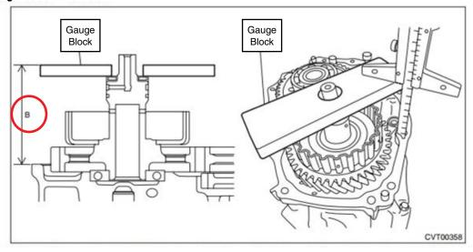
Obtain the thickness of transfer driven gear shim using the following formula to select zero to three transfer driven gear shims.
