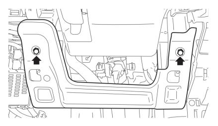
• With the wheels pointed straight ahead and using a hexagon wrench (or equivalent) wrapped with protective tape, locate and press on the snap pins to release the locks (three locations) securing the driver's airbag module.
