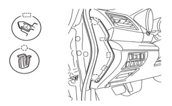
• Remove the data link connector from the lower instrument panel cover, release the 3 retaining clips and remove the lower the instrument panel under cover.
