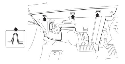
Remove the necessary screws, release the claws and disconnect the harness connectors from the panel's switches before CAREFULLY removing the instrument panel lower trim cover.
