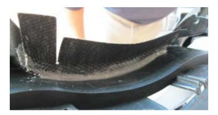
• <u>VERY CAREFULLY</u> using the molded-in groove as a guide, trim the IP as shown to gain access to the square hole for the combination meter top retaining screw clip. After cutting, peel away the trim surface then the foam underneath it to access the square hole for the clip.
