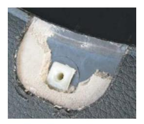
• Along the front edge, (closest to the windshield), there are 2 places where the insulation is heat-fused to the IP. Using a sharp scissor, cut the fuse points off the insulation and use tape to secure it to the new IP as shown below.
