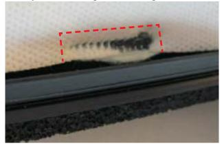
• There is a small piece of fabric-type material which acts as a "cover" for the gap between the top of the steering column and the underside of the combination meter area of the IP. This small trim piece must also be <u>VERY CAREFULLY</u> removed and transferred to the new IP. A small hobbyist knife or equivalent carefully worked in between the material and IP to break the glue bond works well. **PATIENCE** is the key!
