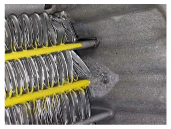
This condition may be the result of excessive thermocycles within the cooling system caused by excessive cycling of the thermostat. These excessive thermocycles within the coolant system may cause the tubes to fatigue, crack and leak at the radiator headers. To correct this condition, a new thermostat has been designed that eliminates the thermostats excessive cycling.
