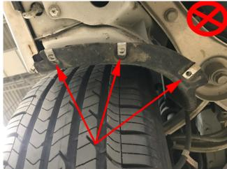
This may be due to incorrect installation of the j-clips installed onto the wheel liner and not onto the sheet metal.
