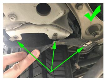
If you encounter a vehicle with the above concern, install the j-clips onto the sheet metal flange as illustrated above and re-insert the 3 screws.
