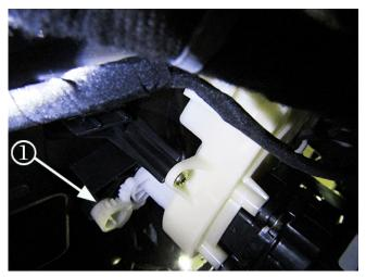
2. From under the IP, locate the driver side floor door gear (1).
