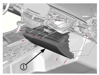
4. Remove the passenger IP compartment (1). Refer to Instrument Panel Compartment Replacement in SI.
