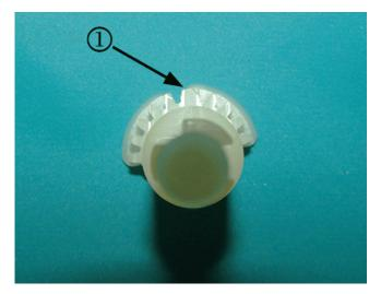
**Note:** In cases where the gear has completely fallen out, it will be necessary to rotate and install the gear in the ONLY orientation where the alignment mark (1) lines up properly to slide past and fully seat into the HVAC case.
