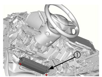
1. Remove the driver IP lower air bag (1). Refer to Instrument Panel Lower Airbag Replacement - Driver Side in SI.
