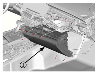
8. Reinstall the passenger IP compartment. Refer to Instrument Panel Compartment Replacement in SI.
