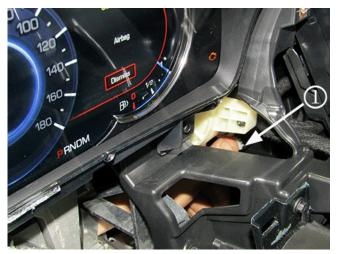
3. Positioning in its proper orientation, reinstall the gear (1). Ensure that the gear is fully seated with the retention feature fully engaged by slightly pulling o the gear. The gear should NOT display any movement.
