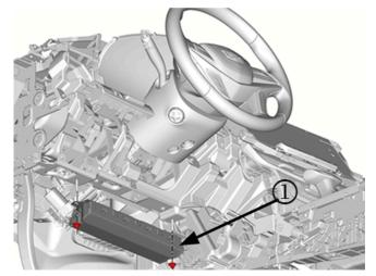
9. Reinstall the driver IP lower air bag. Refer to Instrument Panel Lower Airbag Replacement - Driver Side in SI.
