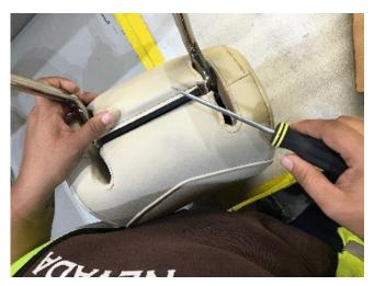
3. Use finger/screw driver to open the J-clip at the bottom of the seat head restraint.
