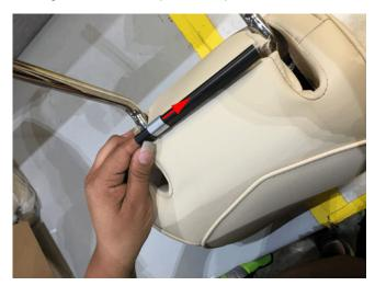
4. Install one metal clip retainer from one side of the J-clip, move it to the center.
