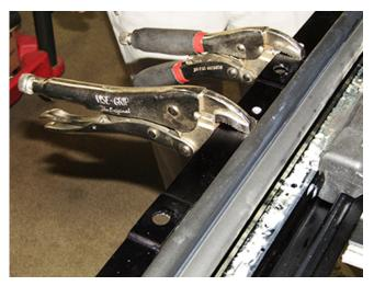
**7.4.** Install vise-grips or a suitable tool, to the housing to hold the metal frame layers in position, while grinding the rivets.
