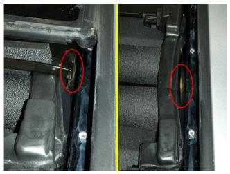
⇒ Inspect the seals for evidence of them being mis-positioned, or rolled out of position on either or both sides. If this condition exists and the guide flange is exposed, there will likely be corrosion evident (shown circled above), due to the metal to metal contact of drain channel to the guide. I exposure of the guide flange or corrosion is evident, continue to step #16.
