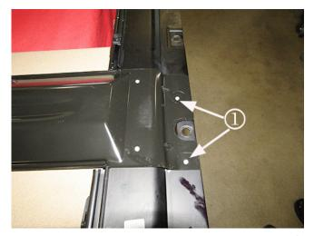
7.3. Locate the two center, outboard rivets (1) on one side of the housing.
