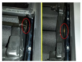
⇒ Inspect the seals for evidence of them being mis-positioned, or rolled out of position on either or both sides. If this condition exists and the guide flange is exposed, there will likely be corrosion evident (shown circled above), due to the metal to metal contact of drain channel to the guide. I exposure of the guide flange or corrosion is evident, continue to step #12.
