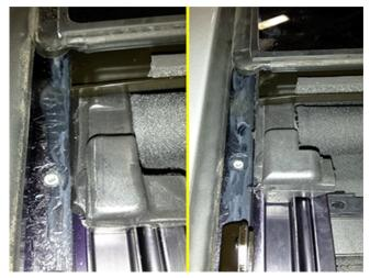
⇒ The graphic above shows examples of proper seal installation. Some slight roll of the seal is acceptable as long as the drain channel is completely isolated from the guide flange. If they are properly positioned on both sides, move ahead to step #13.
