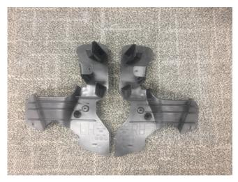
Only install the front lower control arm plastic brake cooling deflector during the PDI process.
