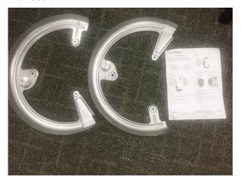
J56 brake cooling ducts and metal wheel blocker rings are intended for track use only.
