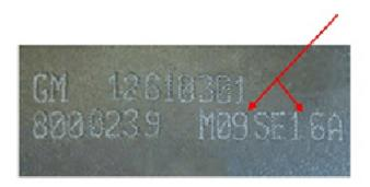
If the vehicle exhibits this condition, remove the starter assembly and inspect for date code correlating with build on date 09/16/2016. The arrows in the code pictured above show the month (9) and the day (16).
