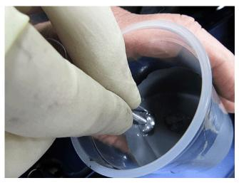
5. Prep the WPC807 rivets by preparing a small portion of catalyzed primer in a mixing cup. Dip the end of the rivet in the primer OR apply a light coat of \*Lloyds Kryptonite Metal Treatment Part Number 36502 with a small brush.
