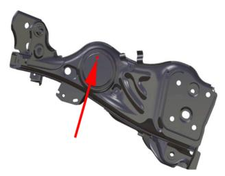
3. Drill a hole with a diameter of 3.3 mm +0.1 (approximately 1/8 inch) in the axle tube end cap on the left and right side of the vehicle in the position illustrated above.
