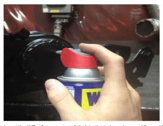
4. Insert the WD-40 spray straw fully into the hole and spray 15 sec. / 25 ml of WD-40 oil per side.
