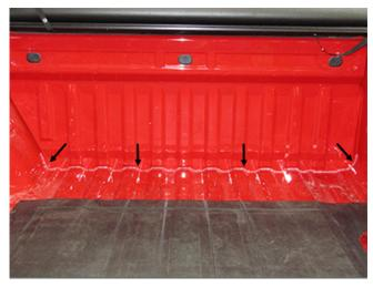
9. Ensure the complete front joint is sealed, and allow to dry per manufacturer's recommendation.
