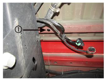
3. Before reinstalling the fuel tank to the vehicle, install one drain hole plug (1) to the open left side drain hole location shown above.
