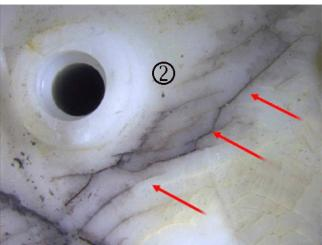
The cause may be sulfuric acid, or other such chemicals, placed in the bed of the truck that has either leaked or been washed through the holes in pickup box, and settled onto the top of the fuel tank. Examples of chemical damage to the fuel pump module such as a fractured port (1) and cracks in the plastic flange (2), are shown in the graphics above.
