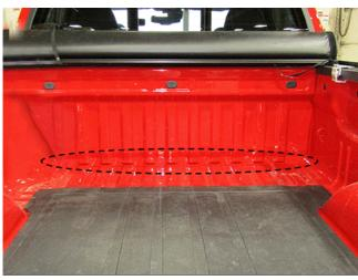
The top side front joint of the pickup bed floor and front panel, shown circled above, is the area that seam sealant will be applied.
