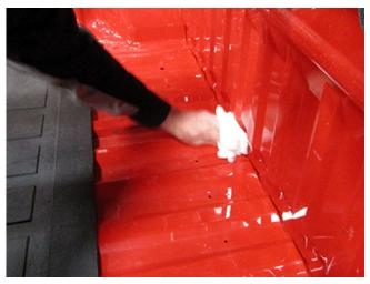
7. Use a rag and wax/grease removing solvent such as Acrysol, or equivalent, to remove any dirt, grease, oil or chemical residue from the repair area.
