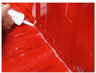
8. Using an appropriate color seam sealer from the table below, or equivalent, apply a bead of sealant across the complete floor/front panel joint.
