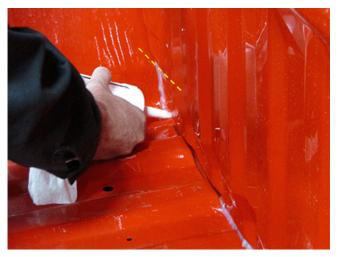
**Important:** As shown in the graphic above, ensure the lower corners are fully sealed by applying sealant past the bottom radius and up to the front panel body line.
