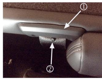
When the front seat is all the way back and the rear 60% seatback is lowered, the added weight of the front occupant puts extra pressure on the seat belt bezel (1) and button/stop (2). This may allow the seat belt to fully retract past the stop, and the retractor may lock because there is not enough seat belt slack to unlock the retractor.
