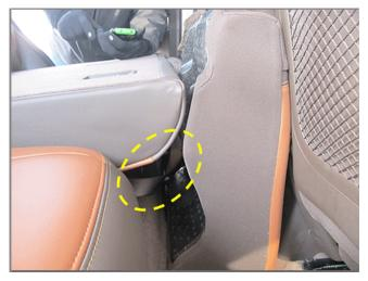
Release the 60% seatback by carefully cutting the rear center seat belt, then replace the rear seat center shoulder belt assembly. Easier access to the seat belt can be attained from the passenger side of the vehicle.
