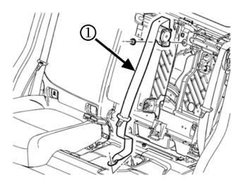
Replace the rear seat center shoulder belt assembly (1). Refer to Rear Seat Center Shoulder Belt Replacement in SI.
