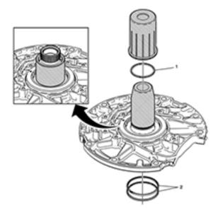
**Caution:** Size the converter fluid seal ring for at least 5 minutes after installation to obtain proper seal ring size. Failure to do so may cause internal transmission leaks and transmission damage.
