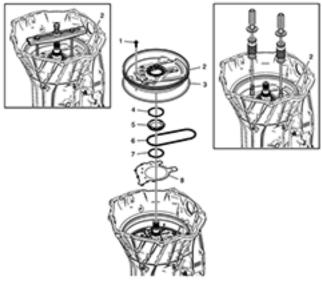
6. Remove the 11 front cover bolts (1). Discard the bolts. The bolts have a dry sealant on them and may only be used once.
