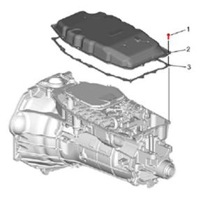
**Note:** The fluid pan gasket is reusable. Inspect the gasket to determine if it may be reused. If the gasket is stuck to the case or pan, it should be replaced.
