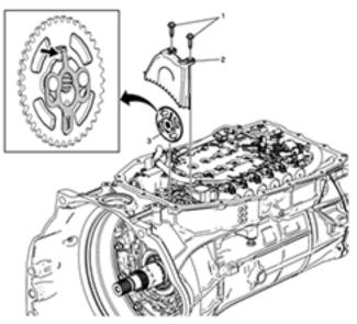
4. Using the DT-48285 Torx Plus socket, remove the two fluid baffle bolts (1) and fluid baffle (2). Discard the bolts.
