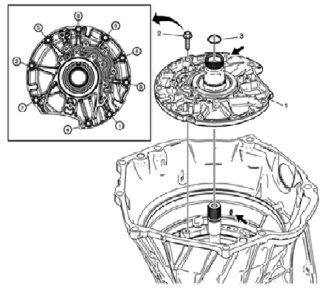
Note: Align the bolt hole indicated by the arrow with the arrow that is cast into the case and push down to seat.
