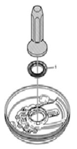
20. Using the *DT*-43772 Torque Converter Seal Installer, install a NEW torque converter fluid seal (1) on the front cover.
