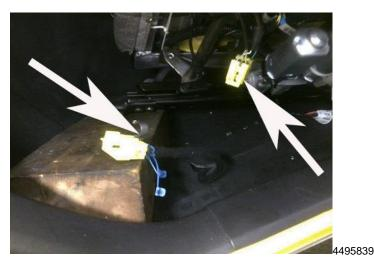
5. Locate the yellow wire connector at the rear cross bar on the seat frame. Remove the connector from the seat cross bar by releasing the metal clip.
