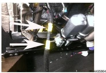
15. Wrap two sections of yellow electrical tape over the polyester electrical tape on both sides of the splice.
