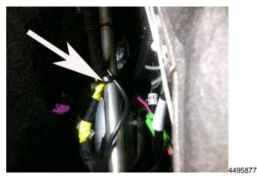
17. Install a wire tie, securing the harness to the seat in the original location. Ensure the wire tie is located on the body side of the wire splice.
