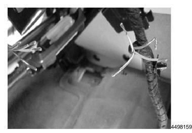
8. Strip off approximately 13 mm (1/2 in) of insulation from the wiring ends. Fold the wires.
