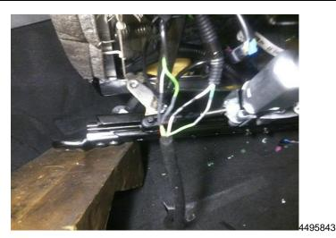
13. Center the heat shrink tube over all four splices and shrink/seal the heat shrink tube securely over the splice crimp and insulated wires.
