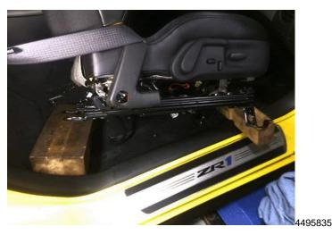
4. Using wood blocks or similar material, tilt and support the seat in the vehicle as shown.
