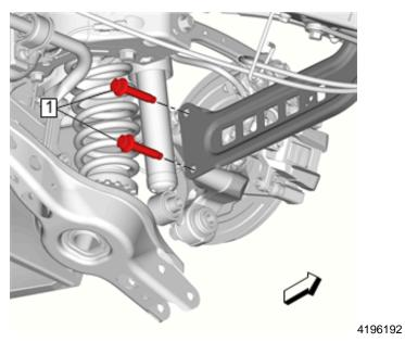
6. Remove the two left trailing arm to knuckle bolts (1). Discard the bolts.
