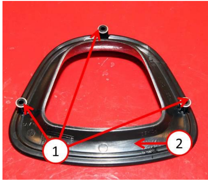
Fig. 2 Install New Wheel Inserts
