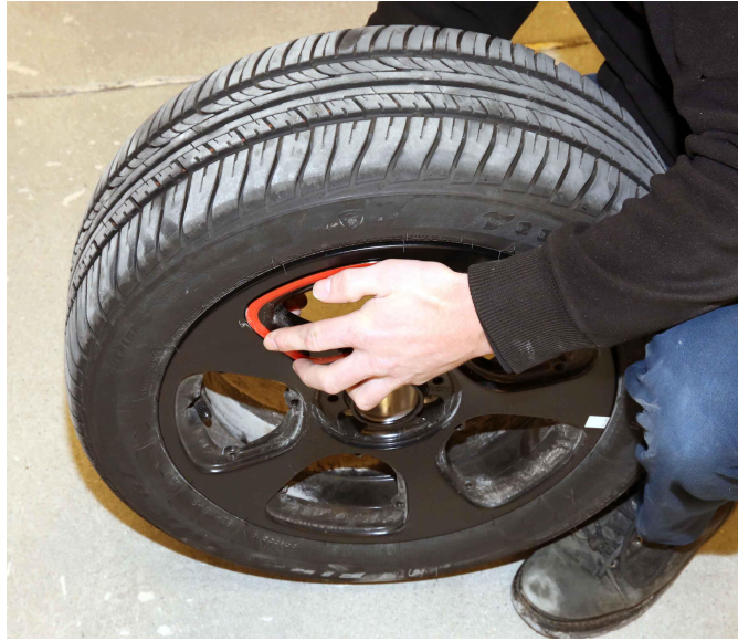
Fig. 4 Install New Wheel Inserts
