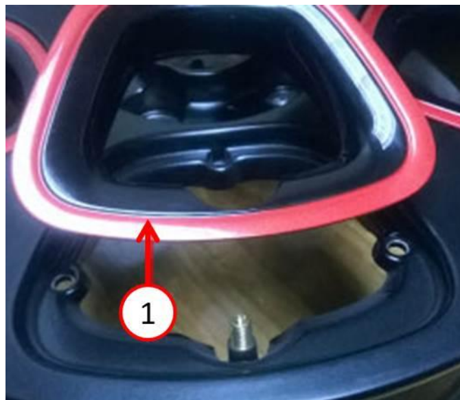
Fig. 3 Place insert onto front of wheel
