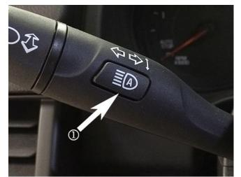
Inspect the turn signal switch and confirm that it is equipped with the auto high beam switch (1).
