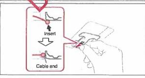
c) Insert the cable end into the inside handle as shown in the figure.
