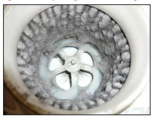
Figure 2. HV Battery Cooling Fan AFTER Cleaning
