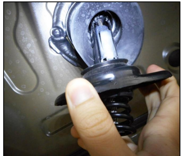
Figure 5. Hook Stuck on the Lip of the Carrier's Housing
