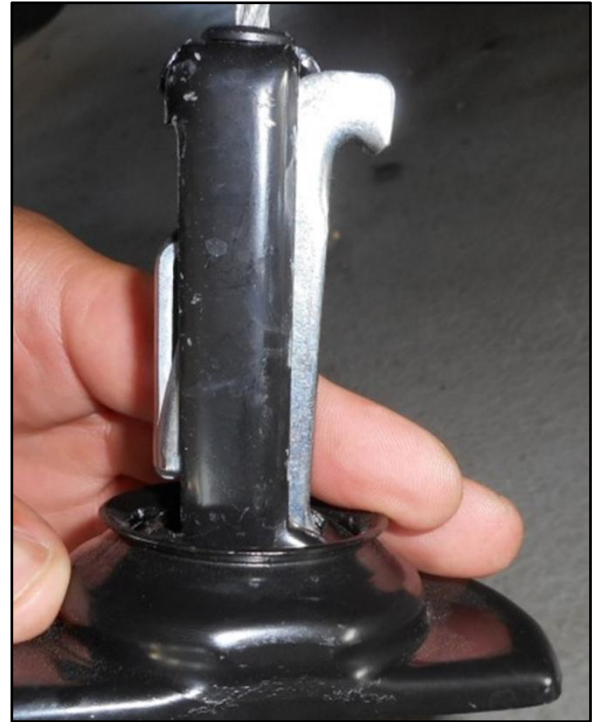
Figure 5. Hook Stuck on the Lip of the Carrier's Housing
