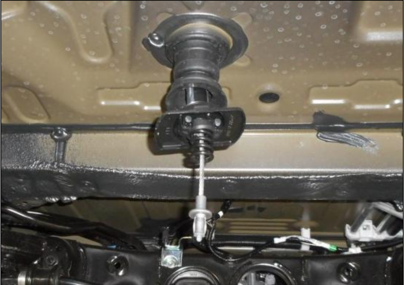
Figure 1. Position of Cable AFTER Spare Tire Carrier Is Stuck
