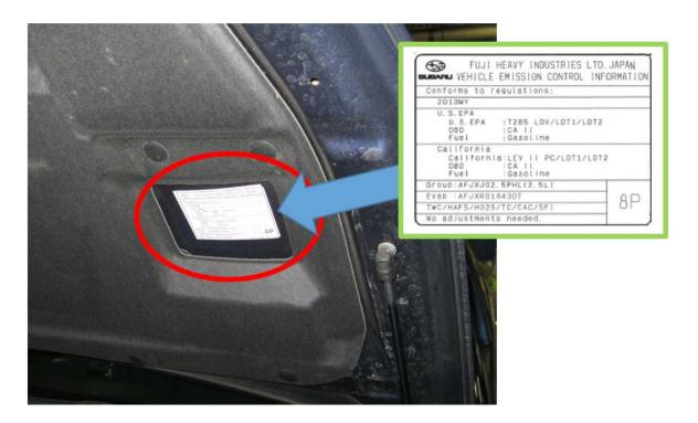
**Step 4:** Use a clean, dry cloth to wipe any dirt or grease from the surface of the original label. **DO NOT** attempt to peel off the original label.
