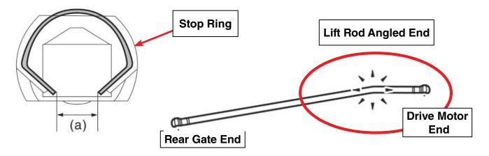
• ALWAYS reinstall the lift rod (angled end downward toward the PRG assembly) **BEFORE** reconnecting the battery. If the PRG assembly were to operate without the lift rod attached, reinstallation of the lift rod may no longer be possible.
