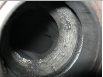
Major Damage to Turbine (Exhaust Side) Housing of the Turbocharger. Turbocharger is recommended to be replaced as an assembly.
