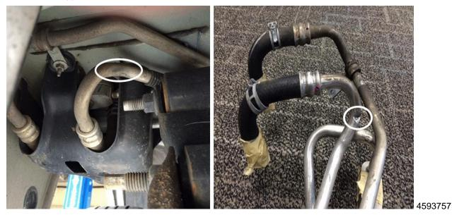
**Note:** If there are any signs of damage to the auxiliary heater hose or evidence of the auxiliary heater hose contacting the spring shackle to leaf spring mounting bolt, the auxiliary heater hose MUST be replaced.
