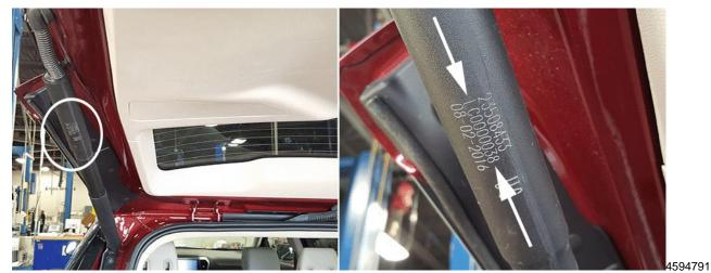
Inspect the second row of the liftgate power assist actuator assembly serial number as shown above. Refer to the Global Connect Reference Library document GCUS-14-709 titled, <u>16046 - Power Liftgate Actuator Serial Number</u> <u>List</u>.
