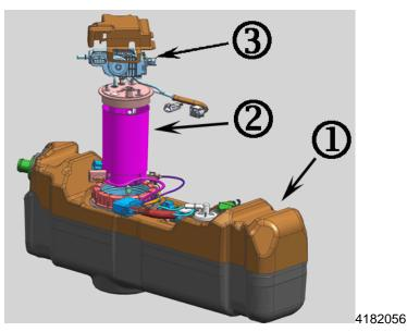
If the Emission Reduction Fluid Tank Reservoir (2) or Pump Module (3) requires replacement in the DEF tank (1), refer to *Emission Reduction Fluid Tank Reservoir Replacement* or *Emission Reduction Fluid Supply Pump Module Replacement* in SI.
