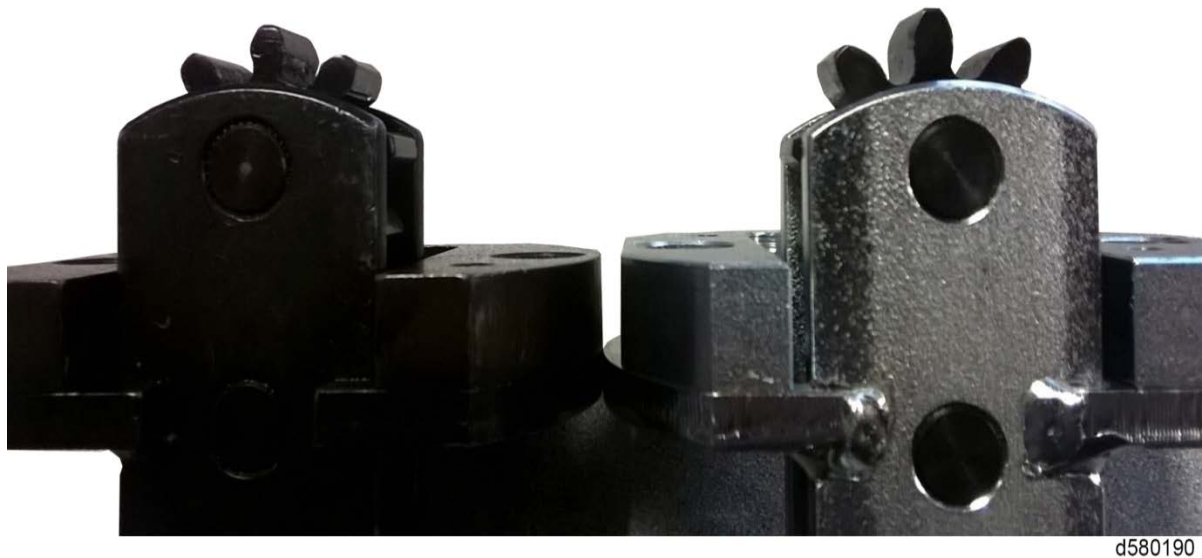
Figure 1. Early Engine Barring Tool (Left) and Later Engine Barring Tool (Right)
