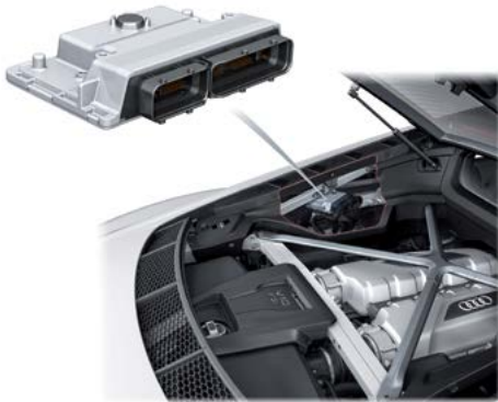
Automatic Transmission Control Module 2 J1006
