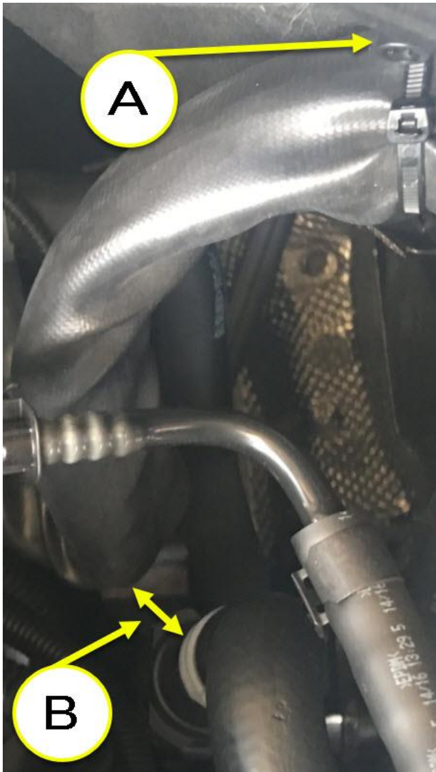
Figure 4. Remove the retaining clip (A) from the firewall and the harness. Place new retaining clip (part number: 3D0971838A) onto the firewall. Position the repair harness so that maintains a 10mm gap (B) between the harness and the coolant pipe. Secure the new retaining clip to the repaired engine harness.
