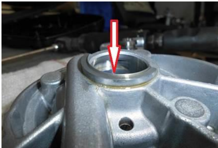
Figure 2) example of worn camshaft bearing bridge
