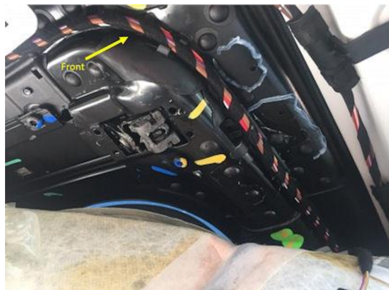
Figure 1 (Water leaking through corner of water channel)
